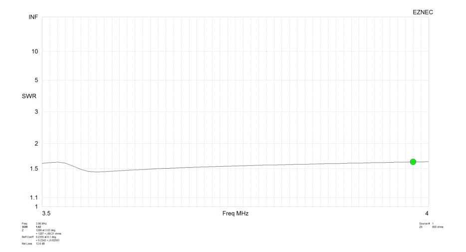
And here with more capacitance for the whole band with 425 pF same position on the leg.
