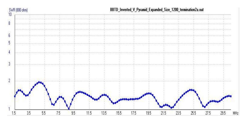
Here is my expanded plot of 75/80 meters for the high end with 175 pF in one leg:
