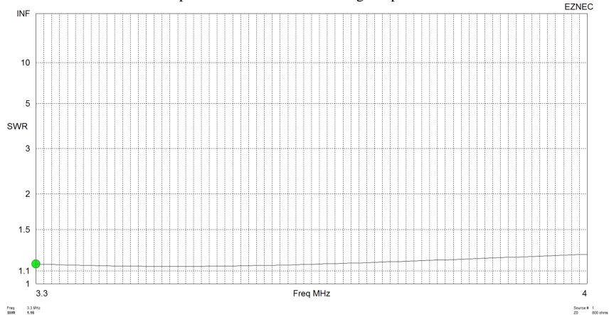
Freq 3.3 MHz SWR 1.16 Z 844.7 at -7.8 deg. = 836.9 - j 114.6 ohms Refl Coeff 0.07337 at -68.17 deg. = 0.02728 - j 0.06811 Ret Loss 22.7 dB
