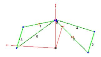
All leg lengths Number 1-6 are 45 feet long and the cross over at the peak number 7,8 are 2 feet. The 1200 ohm termination is on the top cross over and the 16:1 balun and feedline is on the bottom crossover.
